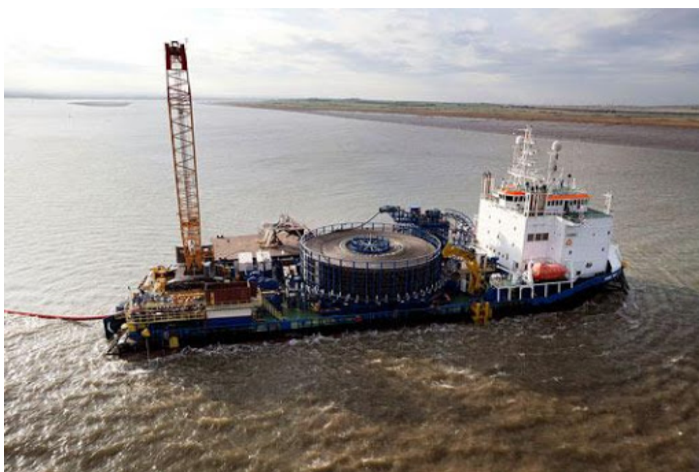
Graphic 4-12 Example export cable installation vessel (Rampion 1 offshore wind farm)
