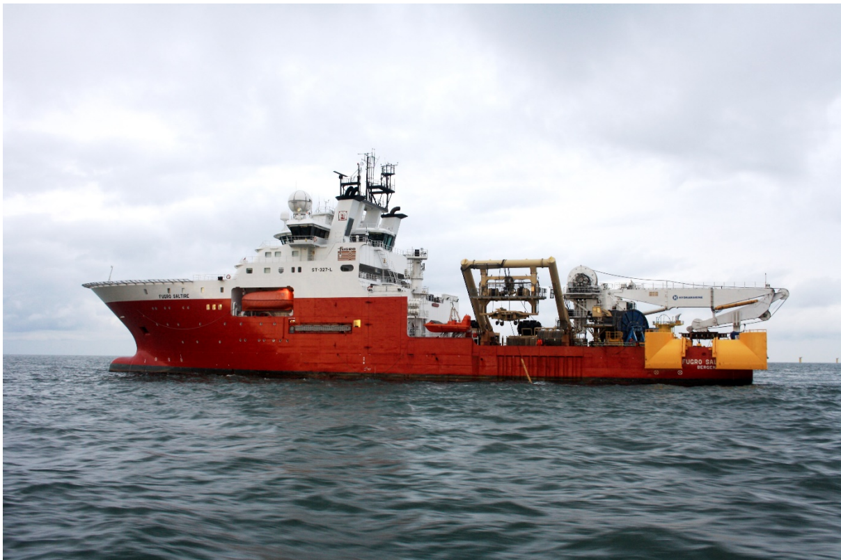
Graphic 4-14 Example cable array installation vessel (Rampion 1 offshore wind farm)
