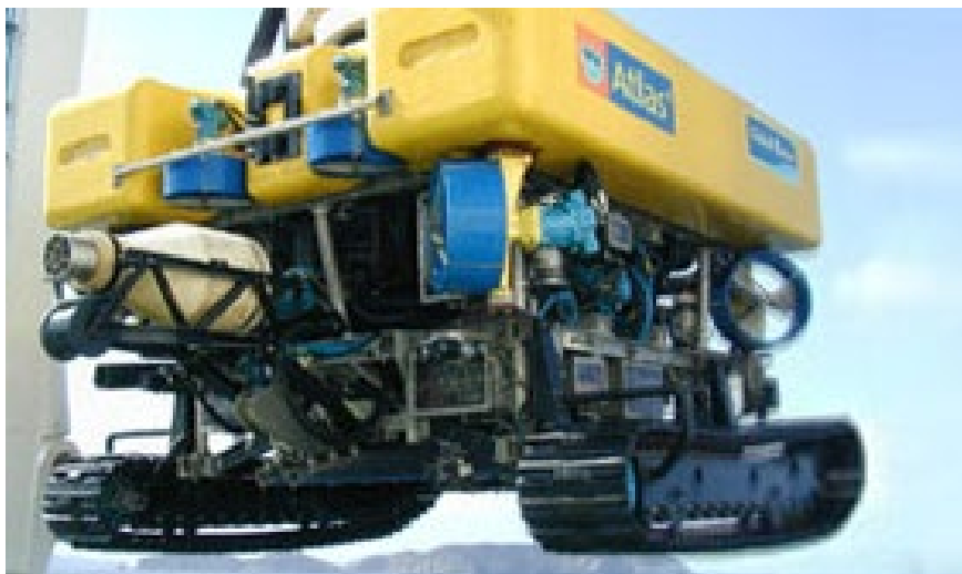
Graphic 4-15 Typical marine cable jetting seabed fluidiser
