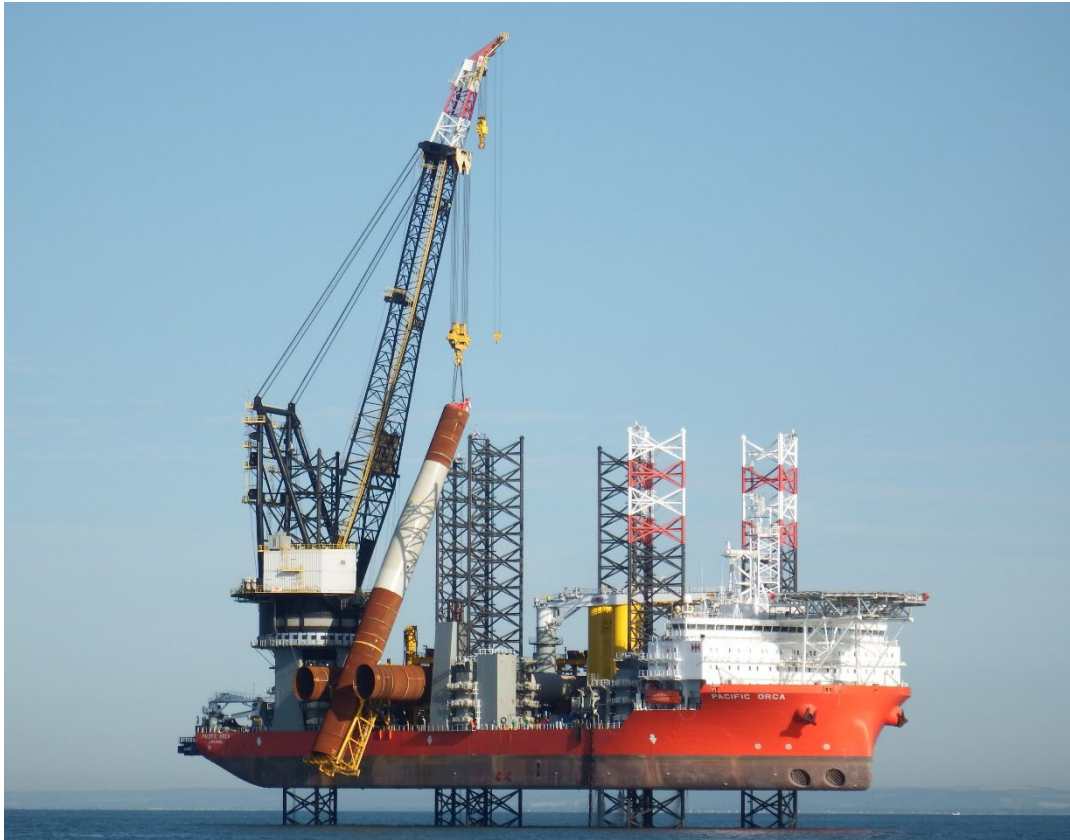
Graphic 4-3 Example jack-up vessel installing a WTG monopile foundation (Rampion 1 offshore wind farm)
