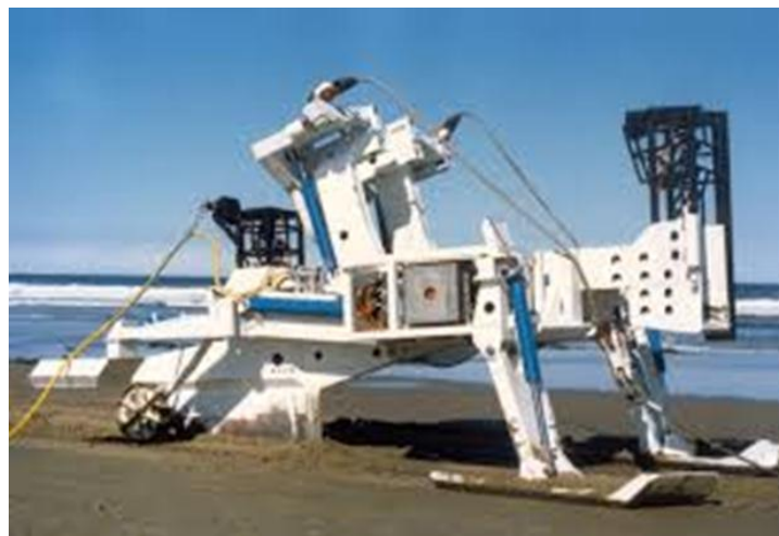
Graphic 4-13 Typical marine cable installation plough
