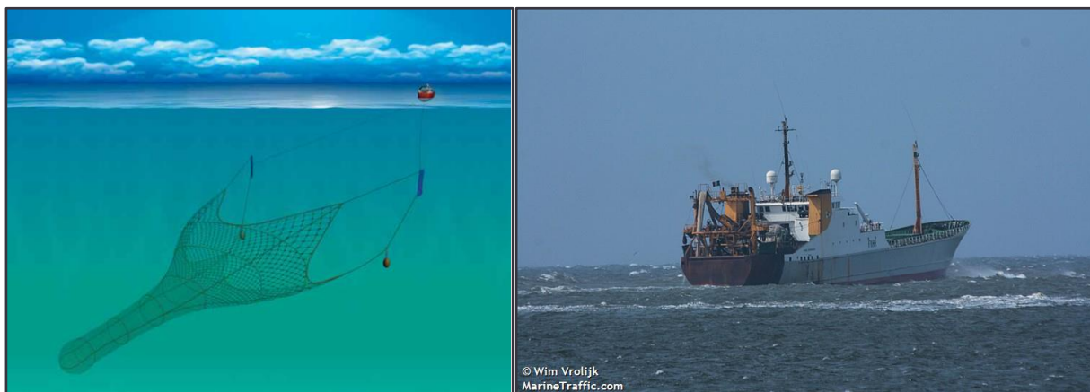
Figure 3-25 Typical pelagic trawl vessel (Source: Seafish, 2015 and MarineTraffic.com, 2020)
