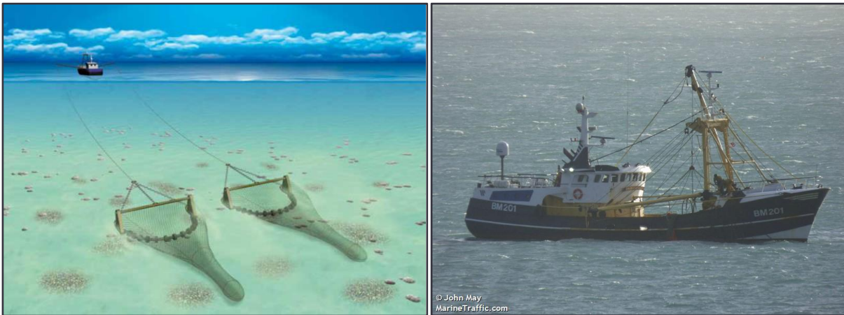
Figure 3-24 Typical beam trawl vessel (Source: Seafish, 2015 and MarineTraffic.com, 2020)
